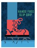
People often get injured when slipping and falling on ice. I created a detachable sole that you can take on and off an existing close-toed shoe, handsfree. This sole incorporates protruded metal spikes that increase traction with ice to prevent accidental slipping.
